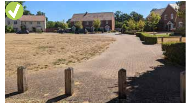
Figure 62: Positive example of well-spaced vehicular barriers of low scale and natural materials that do not obstruct movement, example from outside the parish.
