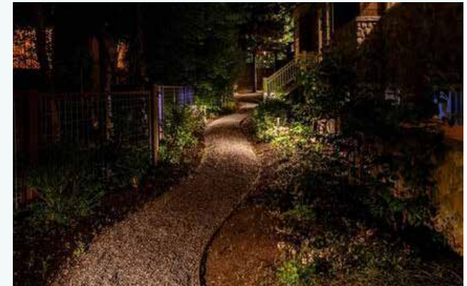
Figure 61: Path-lighting: Use of low fixtures which direct illumination downward and outward.
