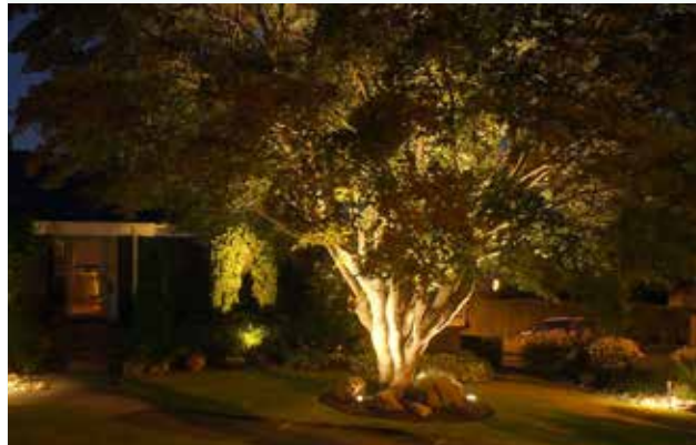
Figure 58: Up-lighting: Focus light and attention on an object or tree from a low fixed location.
