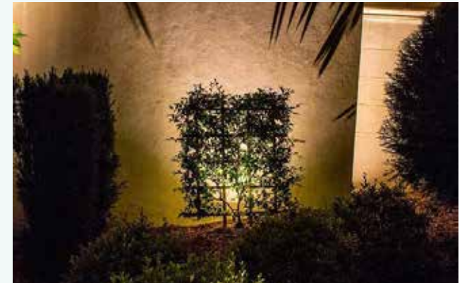
Figure 59: Back-lighting: Fixtures placed at the back of an object to create a 'glowing' effect.
